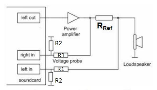
Impedance measurement using a power amplifier.
